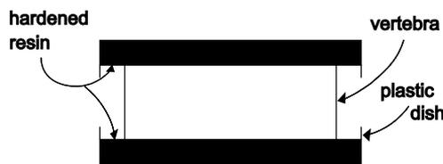
**Figure 2.** Vertebral test construct.
